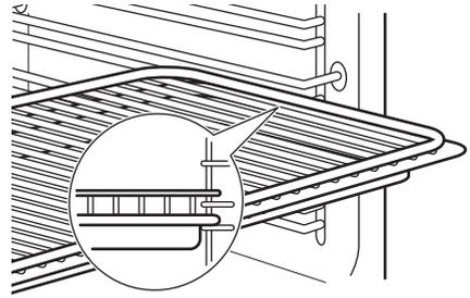
**i** Small indentation at the top increase safety. The indentations are also anti-tip devices. The high rim around the shelf prevents cookware from slipping of the shelf.
