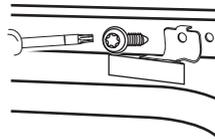
Screw back the screw into the hole after removing the child lock.
