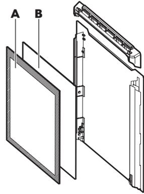
Make sure that you install the middle panel of glass in the seats correctly.
