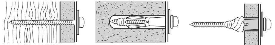
The plugs and screws that come with your IKEA product can be used with most solid and hollow walls. For solid wood walls, use the screws without plugs. If needing additional screws
